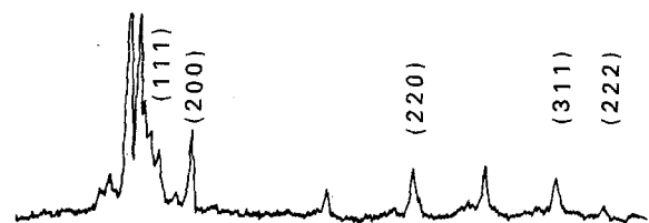
Figure 5 X-ray diffraction pattern of the specimen held at 600°C for 30 min.
